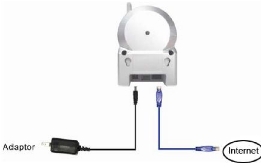
3.IP Camera connection diagram.
